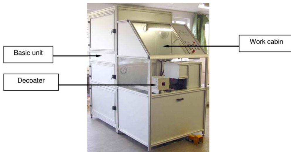
Standard system with a rectangular decoater and double rotating brushes
