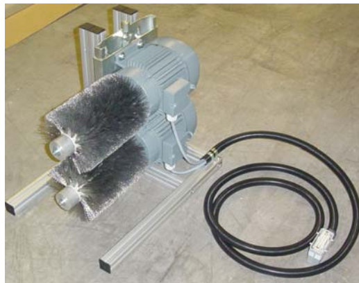
Brush unit without housing, showing the two rotating brushes
