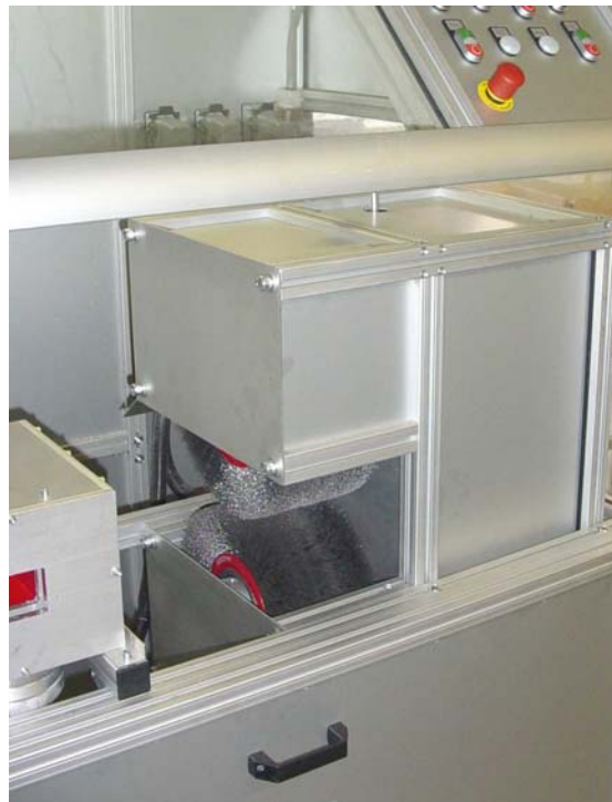
Integrated brush unit with two rotating brushes
