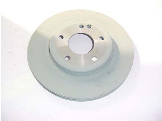
Brake disc before eddy-current decoating Brake disc after eddy-current decoating
