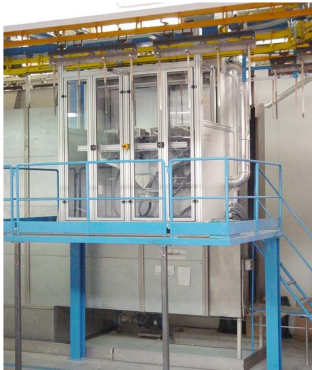
Online process unit parallel to main conveyor
