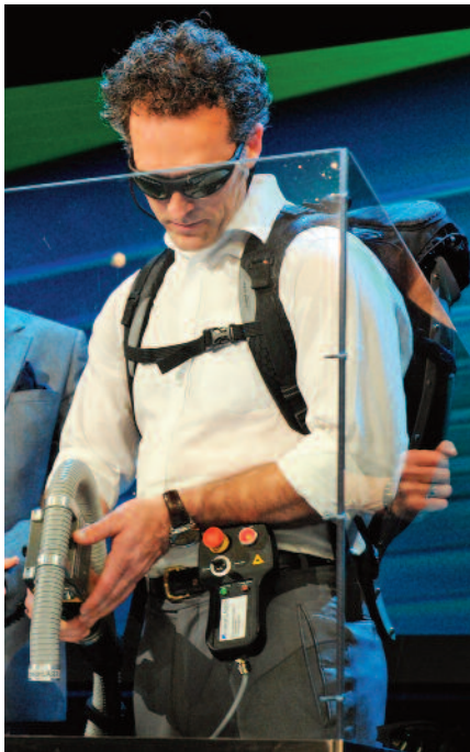
Backpack Laser in action – battery operated - no external power necessary, fiber optic beam delivery, integrated control & cooling unit
