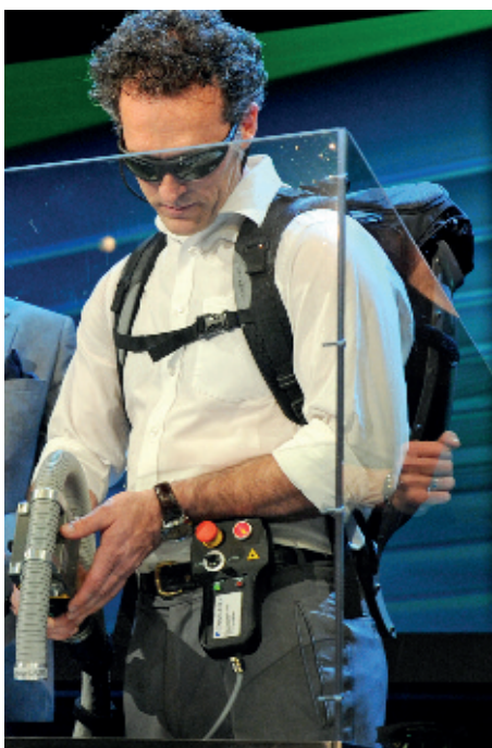
Backpack Laser in action – battery operated - no external power necessary, fiber optic beam delivery, integrated control & cooling unit
