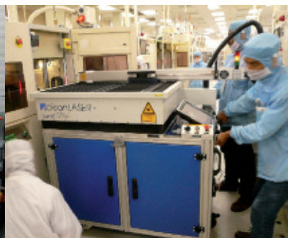
Customized solution "mold WIPER" for cleaning sensitive molds in semiconductor industries
