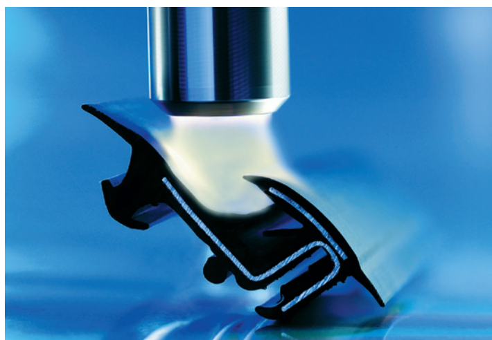
Illustration 4 Pretreatment filling up a crack by means of a jet.
