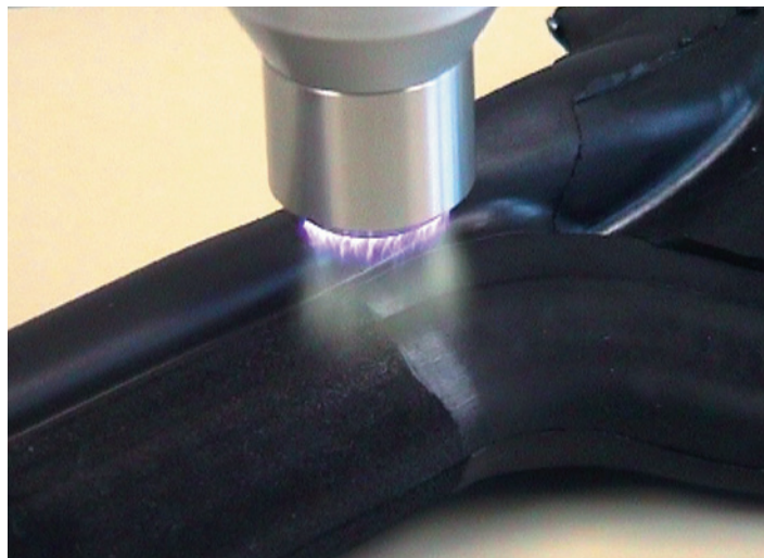
Illustration 3 Frame pretreatment by means of a rotating plasma jet
