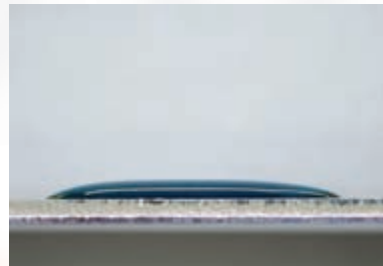
Water drop on plasma treated metal
