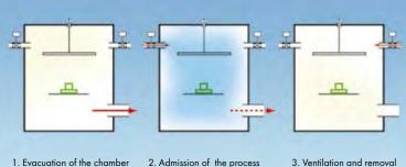
gas and ignition of the plasma 3. Ventilation and removal of the workpieces
