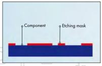
Component with etching mask before plasma treatment
