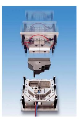
After applying the necessary fusion heat to the plastic part, the feeders move as far apart from each other so that the heating element can move from the working position to the park position.
