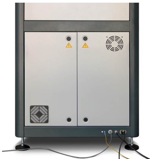
Electrical cabinet at the back of Turnkey M cooled by air and with two wing doors. Electrical and pneumatic supplies are situated at bottom below electrical cabinet.
