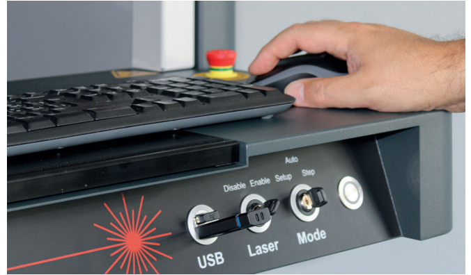
USB ports for memory stick or additional peripherals like mouse or keyboard.
