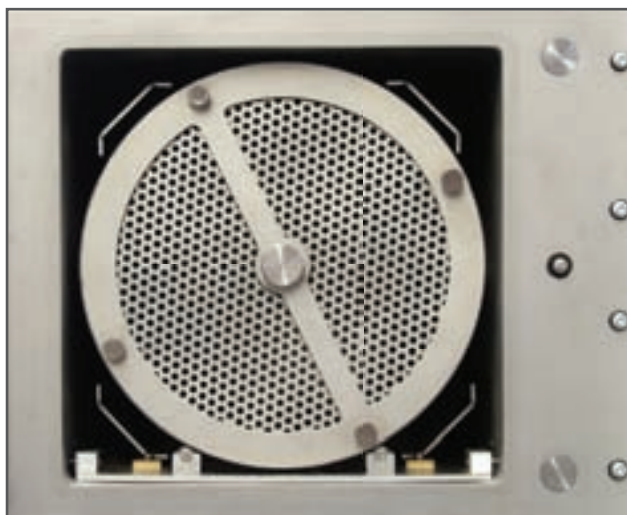
Pics: Removable rotary drum for Tetra 150
