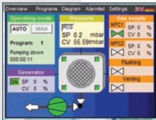
PCCE Control (Windows CE) / PCCE Steuerung Software (Windows CE)
