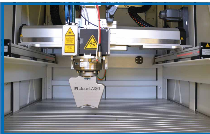
cleanCELL-portal with shareMOTION-optic for efficient adhesive pre-treatment
