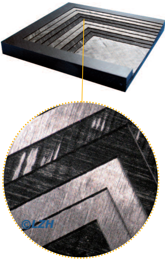
Figure 1: Laser based machining of stepped structure (ply-by-ply ablation) for bonded repair
