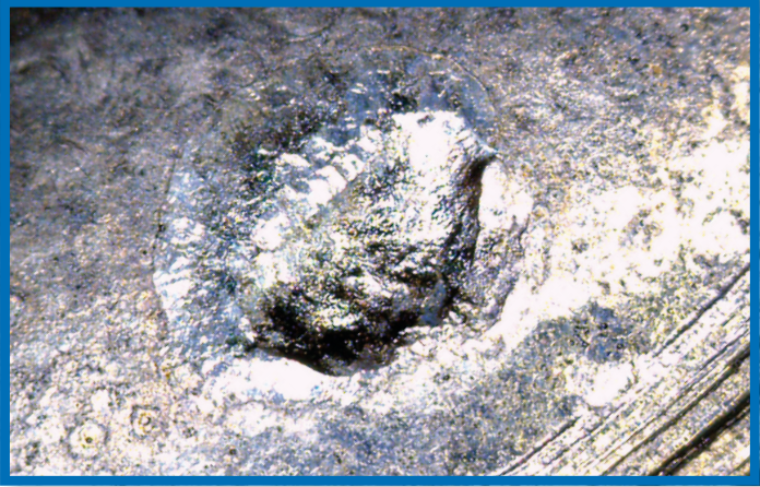
Part after welding post-treatment by cleanLASER; silicate residues completely removed
