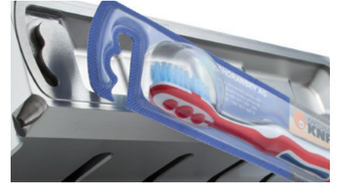
Format-dependent blister pack with sonotrode
