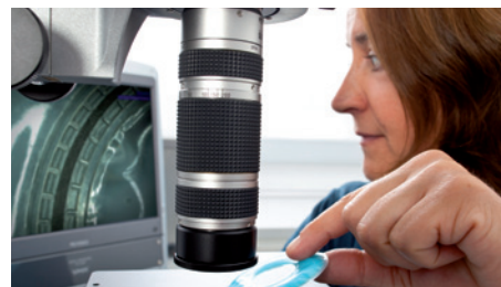
Inspection of the sealing seam in the test laboratory
