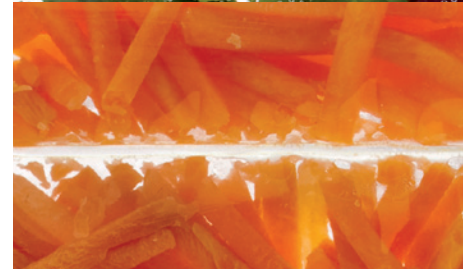
Sealing through areas in contact with the product
