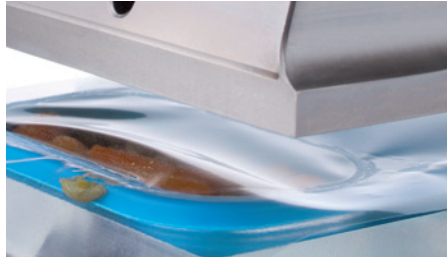
Sealing a tray in contact with product
