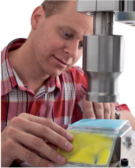
Combined sealing and punching
