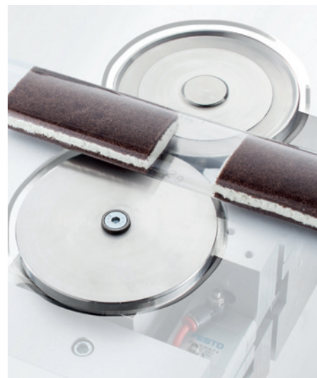
Ultrasonic sealing of fin seams with the one side mounted roll seam module
