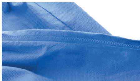
Ultrasonic roll seam welding of OT clothes
