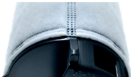
Ultrasonic roll seam welding of filter fabric on a plastic core
