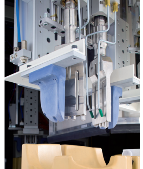
Ultrasonic units for riveting airbag covers
