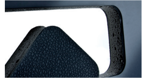
Punching composite materials (Slush/PUR/ABS)
