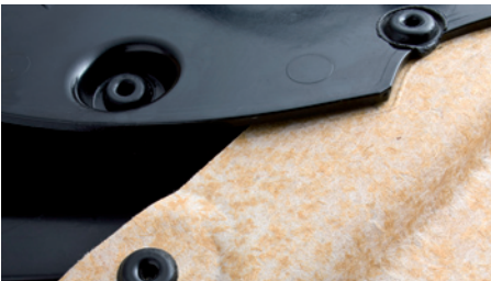
Riveting points of a passenger car door
