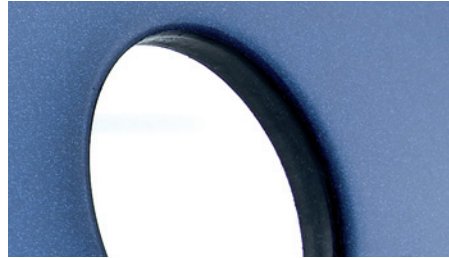
Paint drawn in during radial embossing
