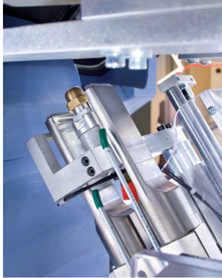
Sonotrode for welding parking sensor holders
