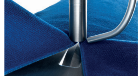
Slitting of fabric with fixed sonotrode
