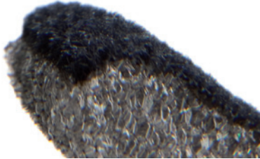
Cross section of cut edge of ultrasonically punched pad
