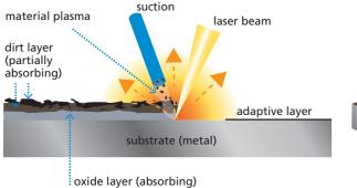
The focused, very short-pulsed laser beam is a media-free method of coating vaporization.
